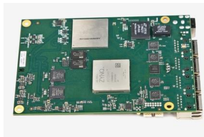
Figure 2-26: digiBackBoard with the cooling and SMA adapters, Bottom and Top view.
