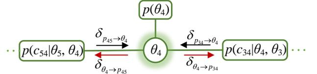
Fig. 5. Message passing in Belief Propagation.
