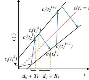
Fig. 2. Message exchange between adjacent nodes.
