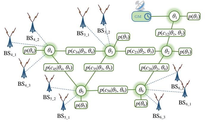
Fig. 4. Factor graph corresponding to an exemplary communication network.
