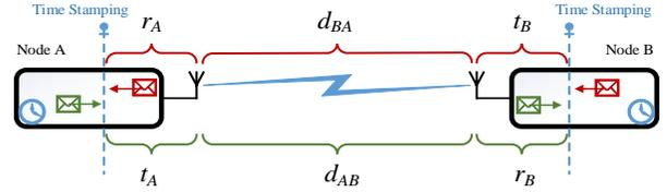
Fig. 1. Delay Decomposition.
